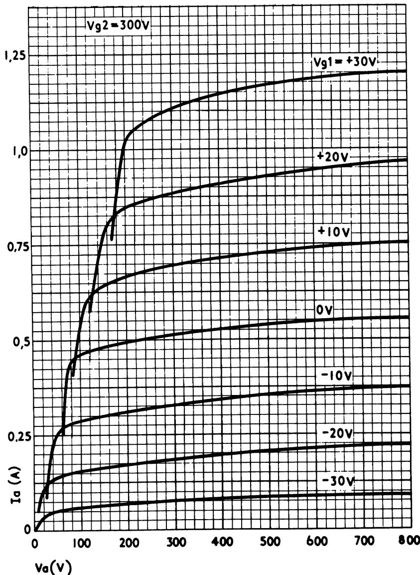
**SCREEN CURRENT – ANODE VOLTAGE. SCREEN VOLTAGE OF 300V
