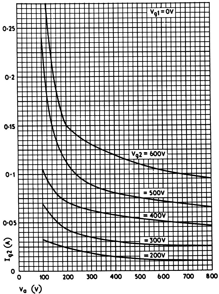
**CONSTANT ANODE CURRENT CURVES WITH SCREEN VOLTAGE AT
