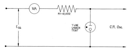
Vary current from 5made to 30made and back to 5made(by adjusting Ebb slowly). Sudden voltage jumps registered on the oscilloscope snall be not greater than the specified value.
