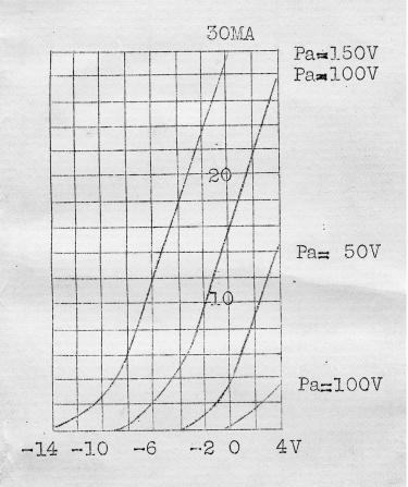
Amplification factor Mutual conductance (max): 3 MA/V 37001L Impedance: 5-8 MA Plate current: Maximum Overall Height 110 m m Maximum " Diameter 50 m m 100 150 Plate Voltage: Negative Grid Voltage: 3-4,7-9, 200 12-14
