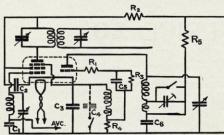
$\begin{array}{l} R_1\!=\!1,\!000~\text{ohms.} \\ R_2\!=\!5,\!000~\text{ohms.} \\ R_3\!=\!50,\!000~\text{ohms.} \\ R_4\!=\!500~\text{ohms.} \\ R_5\!=\!50,\!000~\text{ohms.} \\ C_4\!=\!0.1~\text{mfd.} \\ C_2\!=\!0.1~\text{mfd.} \\ C_3\!=\!0003~\text{mfd.} \\ C_4\!=\!.001~\text{mfd.} \\ C_5\!=\!.0005~\text{mfd.} \\ C_6\!=\!0.1~\text{mfd.} \end{array}$
