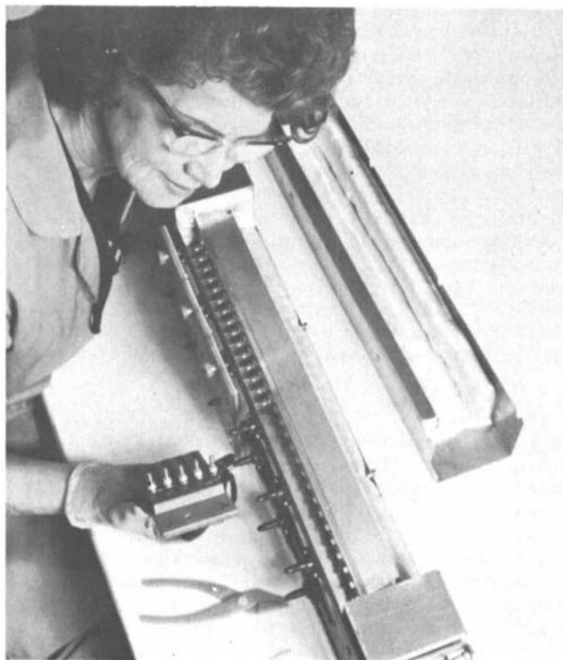
Fig. 35 Life-test block for type-10A transistors
