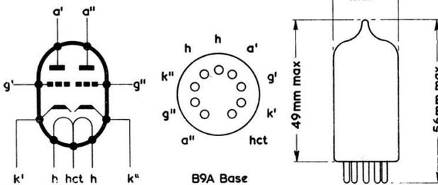
The bulb and base dimensions of this valve are in accordance with BS448, Section B9A
