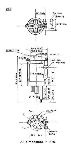
Mechanically-tuned klystron of all-metal construction designed for use as a local oscillator over the frequency range 8702 to 9548 Mc/s.
