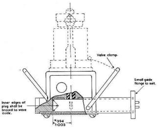
Dimensions indicated by a determine the broad band characteristics of the coupler and should be held to tolerances shown.
