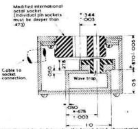
Dimensions indicated by & determine the broad band characteristics of the coupler and should be held to tolerances shown.
