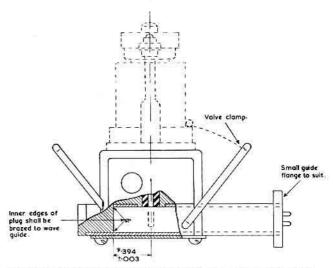
Dimensions indicated by # determine the broad band characteristics of the coupler and should be held to tolerances shown
