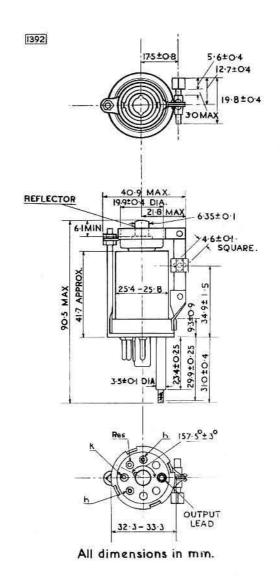
Mechanically-tuned klystron of all-metal construction designed for use as a local oscillator over the frequency range 8500 to 9660 Mc/s.
