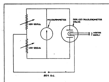
Recommended bridge circuit for use with the DDR.100
