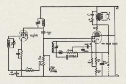
Efficient filtering of H.F. from the pentode will lead inevitably to some attenuation of the higher audio frequencies and the condenser in the anode impedance limiting circuit may with advantage be reduced to a smaller value than that usually fitted.
