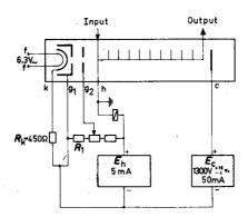
Designations of the grids: g<sub>4</sub> = focusing electrode (Wehnelt) g<sub>2</sub> = acceleration electrode
