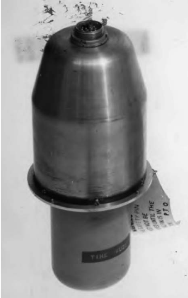
FIGURE 7 The clockwork fuze. Delivery problems with the clockwork jeopardized Britain's strategic deterrent. Shortcomings in the cocking mechanism that wound the fuze led to premature detonation, a problem resolved with extra washers to eliminate asymmetry in the winding plunger.
