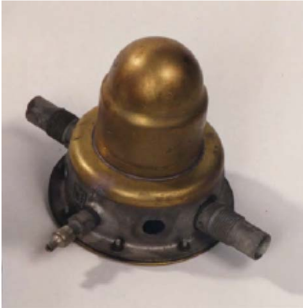
FIGURE 8 Bridge wire detonators assembled by banks of women at Woolwich. They were ‘potted’ in a material akin to plaster of Paris. Crown copyright 2013, with permission
