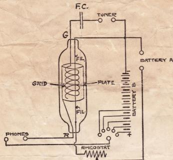
series. It is very important that each shows at least  $3\frac{1}{2}$  volts to  $4\frac{1}{2}$  volts and that they are properly connected together. are proper-ed together, ly connected together, otherwise the results will be very poor. The negative or zinc end of this battery must lead to the filaconnected ment.
